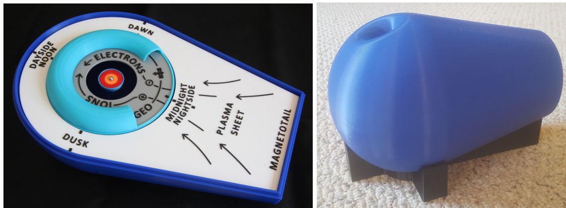
Plasma_Sheet inserted into assembly (left). Magnetosphere_Upper_Half fits over full assembly (pictured with stand, right).
