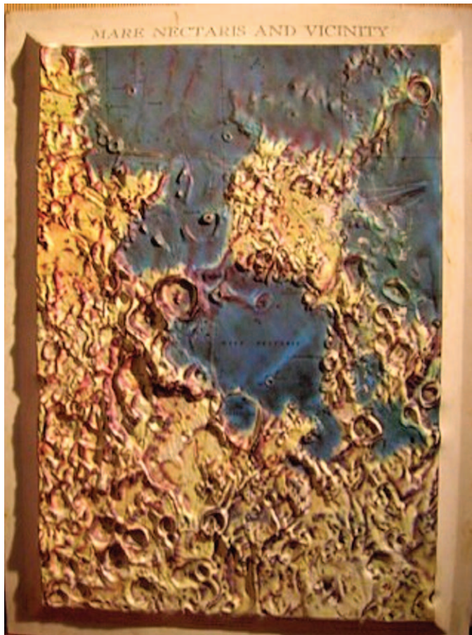
FIGURE 1: Relief map of the Mare Nectaris region of the Moon, constructed by the Army Map Service in 1961 based on telescopic observations. Similar (but much higher resolution) base-relief maps were later constructed from each Apollo landing site.
